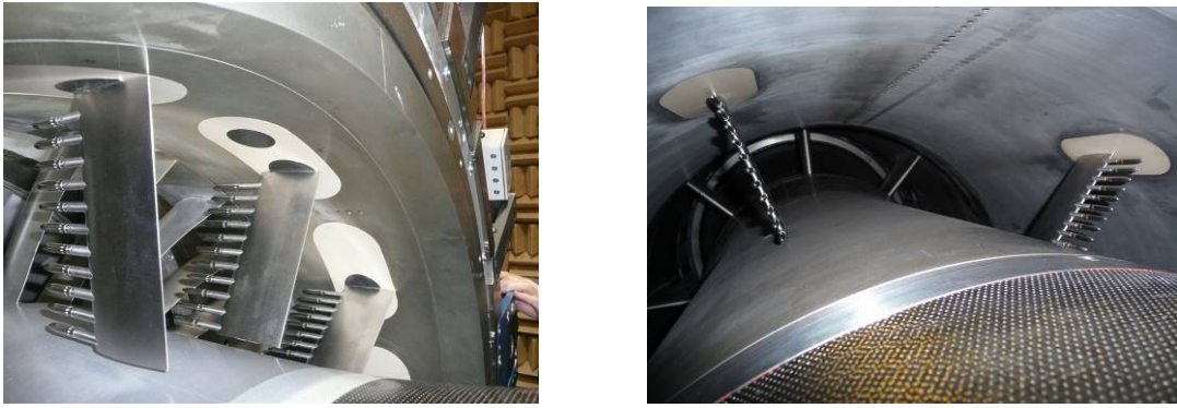
Fig. 6: Sensor rakes RMD1 at OGV exit (left photo). Sensor rakes RMD2 and axial sensor array RMD 3 at nozzle equivalent plane.
