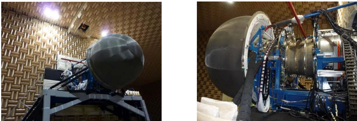
Fig. 1: UFFA rig installed in the anechoic test facility of AneCom AeroTest.
